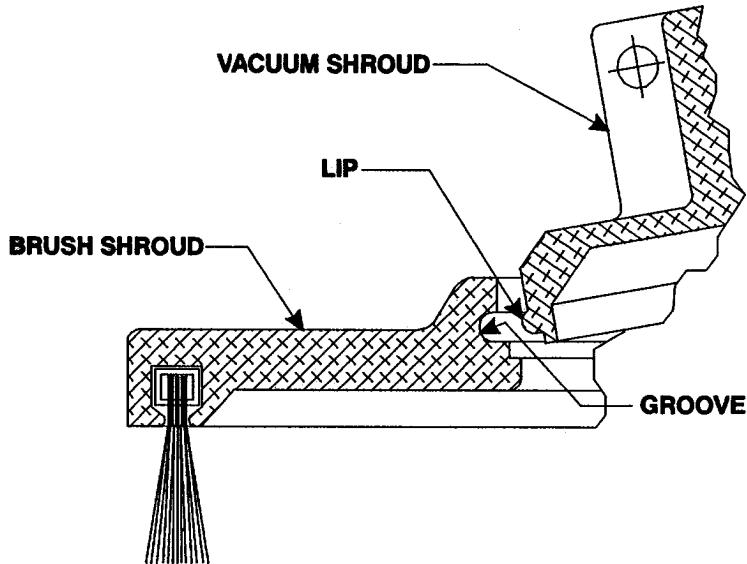
2. Do not rest tool on the brushes. This will cause them to bend and "Take a set" reducing pick-up efficiency. Store tool on its back when not in use.
